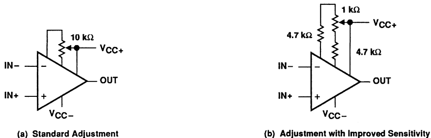
Figure 47. Input Offset Voltage Nulling Circuits
