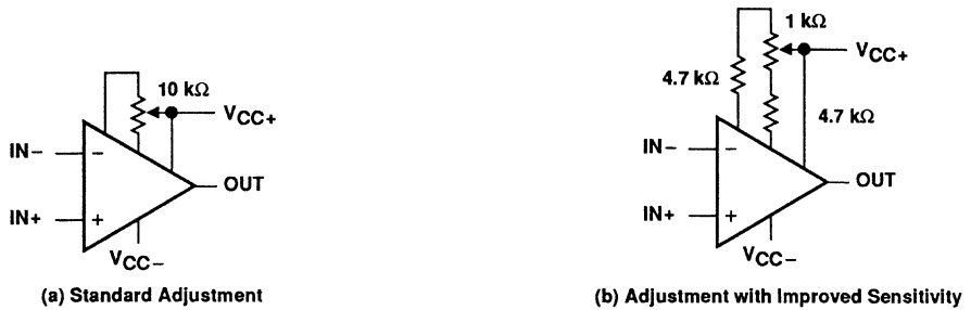
Figure 44. Input Offset Voltage Nulling Circuits
